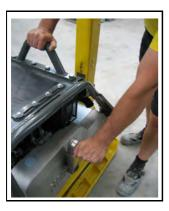
5. Hold the crank handle with one hand, and support the protective cage with the other.
