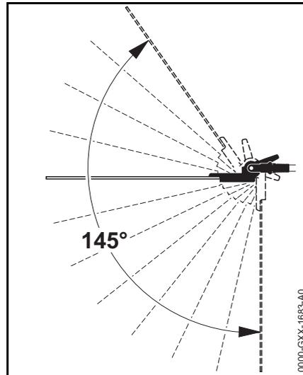
The angle of the cutter bar can be adjusted upwards in 4 stages from 0° (straight) to 55°, and downwards in 7 stages from 0° to 90° (right angle facing down). There are therefore 12 possible working positions.
