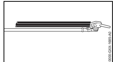
The cutter bar can be folded flat against the drive tube and locked in position to save space during transportation.
