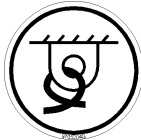
Fig. 8: Label for points used for tying down the machine
